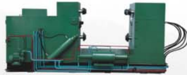
YFS-Z型 液压阀门试验台 (高低压水泵) High and Low Pressure Water Pumps of Hydraulic Valve Test Bench of Model YFS-Z
