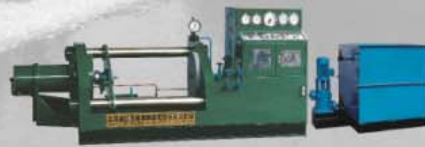
YFS-D型 液压调节阀试验台 Hydraulic Control Valve Test Bench of Model YFS-D
