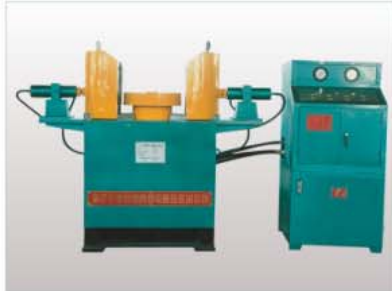
YFS-M型 液压阀体毛泵试验台 Hydraulic Roughcast Valve Body Test Bench of Model YFS-M
