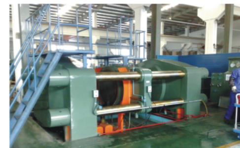
YFS-D2200型 液阀门试验台 ( 用于试压大口径、高磅级球阀、抽气截止阀等 ) Hydraulic Valve Test Bench of Model YFS-D2200 (for Testing Large Size and High Pressure Ball Valves, Extraction Check Valves etc.)
