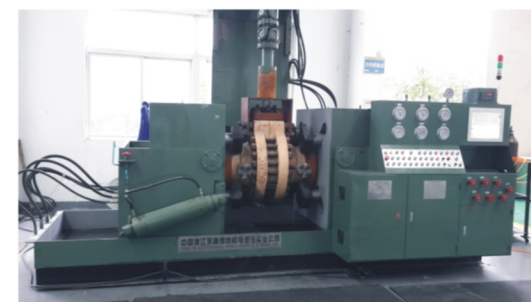
YFS-Z500型 智能型液阀门试验台 ( 用于阀门压力性能测试和扭矩测试 ) Intelligent Type Hydraulic Valve Test Bench of Model YFS-Z500 (for Testing Valves' Pressure Performance and Torque)
