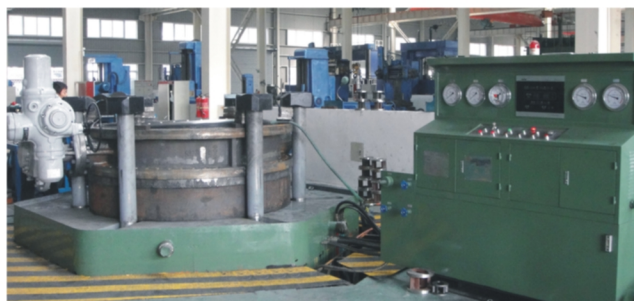
YFS-DL3000型 液阀门试验台 ( 用于试压大口径蝶阀 ) Hydraulic Butterfly Valve Test Bench of Model YFS-DL3000 (for Testing Large Size Butterfly Valves)
