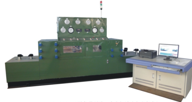
YFS-A100/300型 智能型液压安全阀试验台 ( 台式 ) Intelligent Type Hydraulic Safety Valve Test Bench of Model YFS-A100/300(Combined Type)
