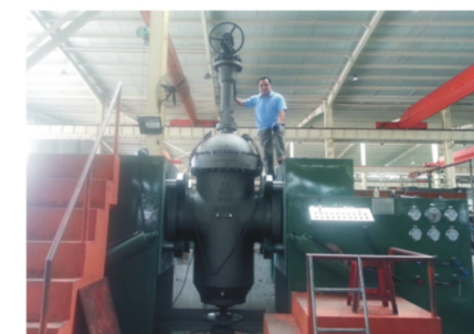
YFS-Z800型 液阀门试验台 ( 用于试压大口径平板阀 ) Hydraulic Valve Test Bench of Model YFS-Z800 (for Testing Large Size Flat Gate Valves)
